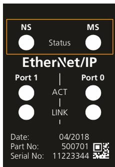
Figure 10: EtherNet/IP™ status LED's
