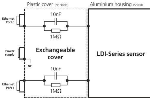
Figure 6: Shielding concept of the LDI-Series sensor and the exchangeable cover with Industrial Ethernet
